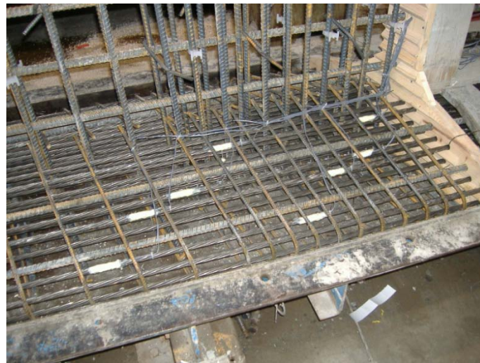
Figure 6- 3: 0.6-in. diameter strands with strain gages staggered over different rows
