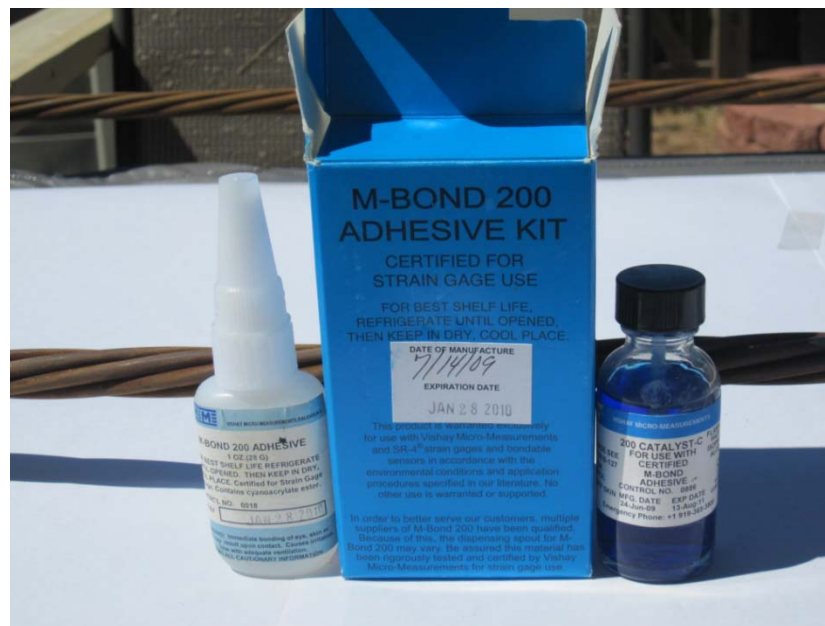
Figure 6-14: M-Bond 200 adhesive kit by Vishay Precision Group (Vishay Precision Group, 2010).
