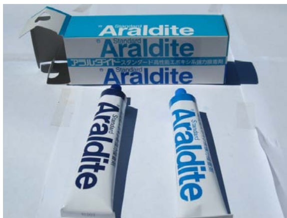
Figure 6-17: Araldite standard coating agent by Texas Measurements, Inc. (Texas Measurements, Inc., 2010).
