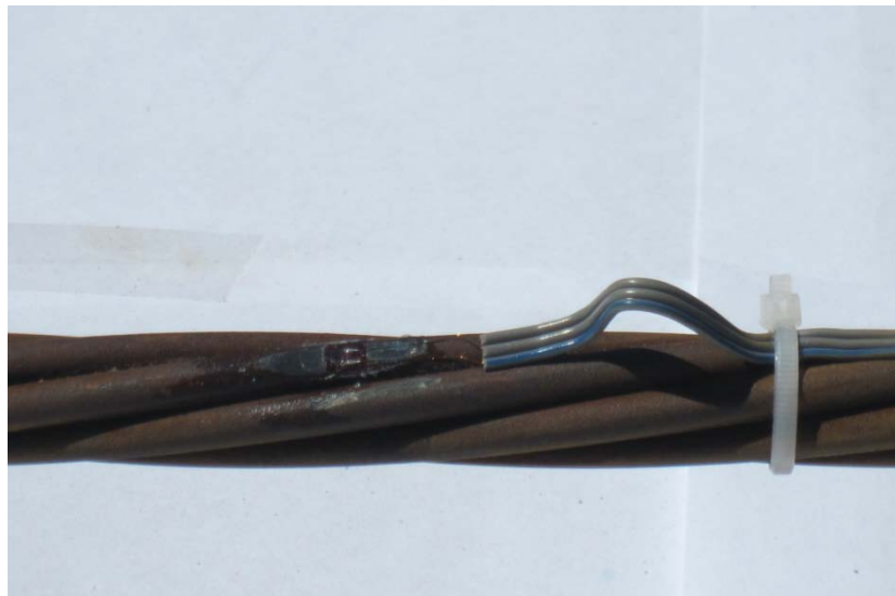
Figure 6-20: Lead wires attached to the strand using a typical plastic strap while allowing adequate slack in the wire adjacent to the gage.
