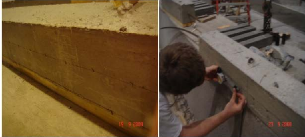
Figure 4-1: Typical experimental specimen with DEMEC discs on the outside faces to facilitate measurement of straining after the release of pretensioning (Akhnoukh, 2008).
