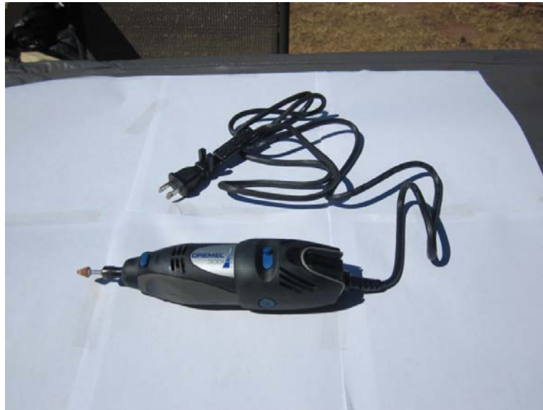
Figure 6-13: A typical hand-held grinder required for surface preparation.
